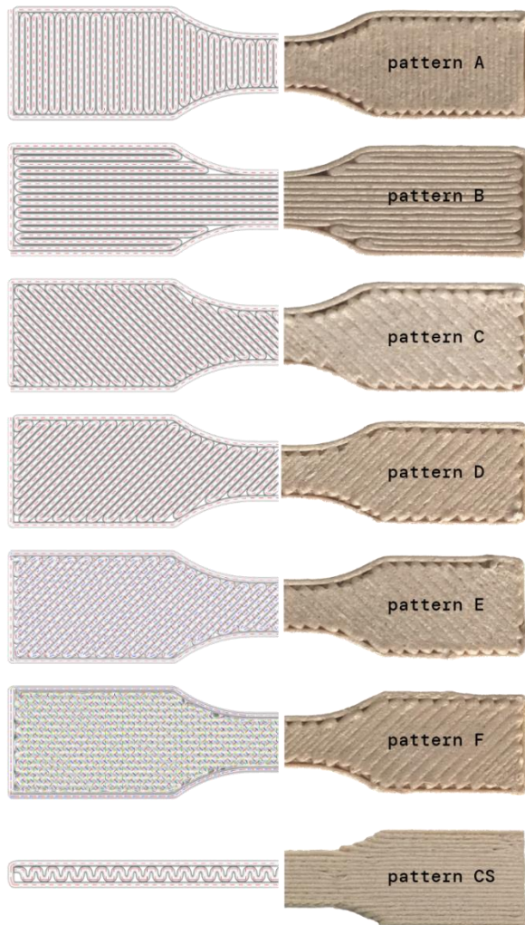
Fig.1. Digital representation (on the left) and photographs (on the right) of the specimens' layering orientation, top view.
