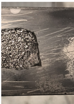
Figure 28 - Damaged carbonized sample based on the water washable resin
