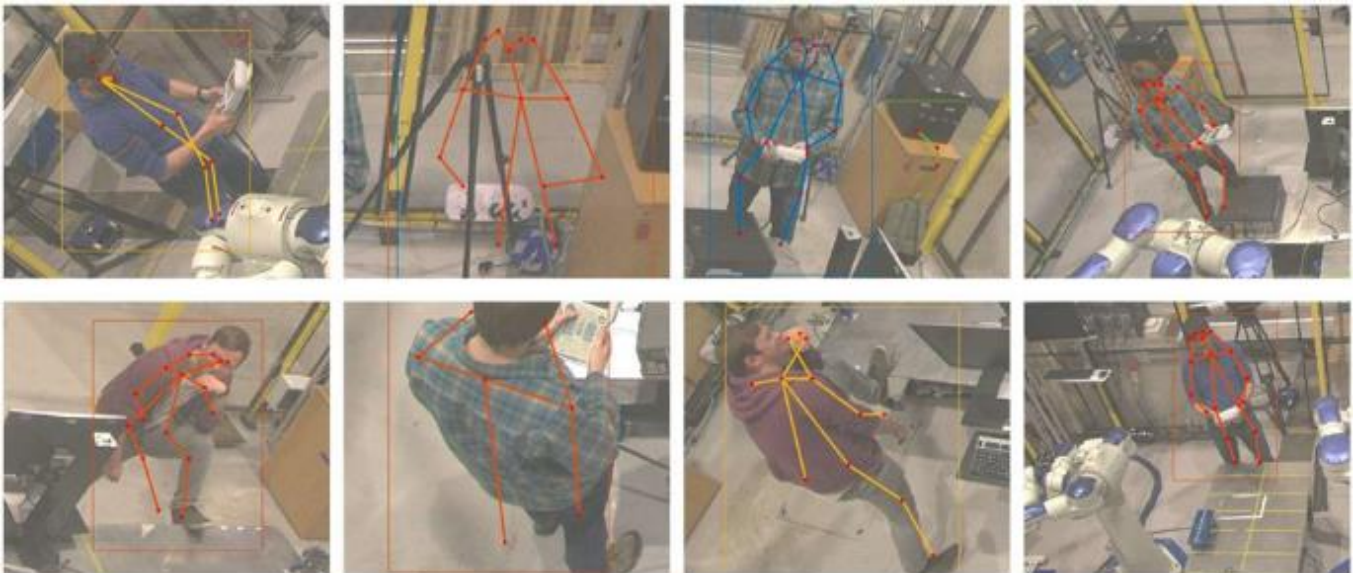
Figure 6 OpenPose tested in the cell. The algorithm detects body parts and connects them creating a skeleton-like structure.
