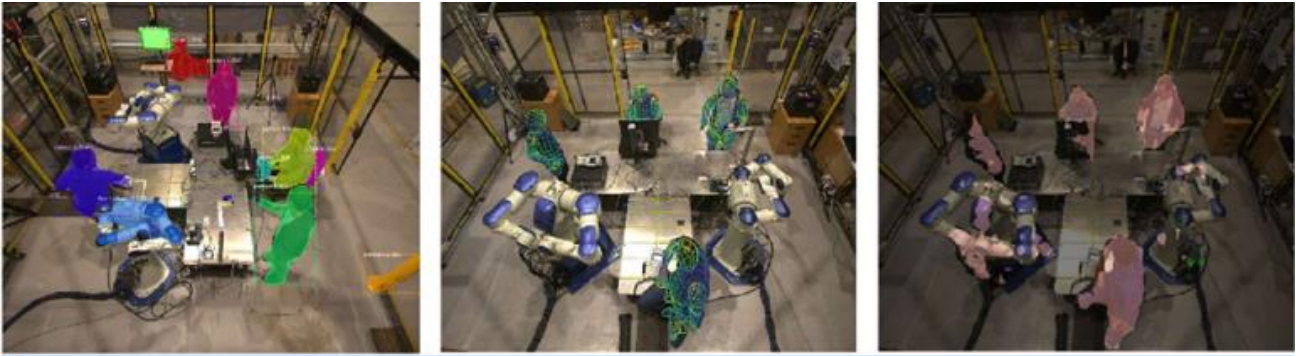
Figure 5. Segmentation algorithms applied to a manufacturing setting. Left: Mask R-CNN [2]; Center: DensePose [4]; Right: DeepLab [1]
