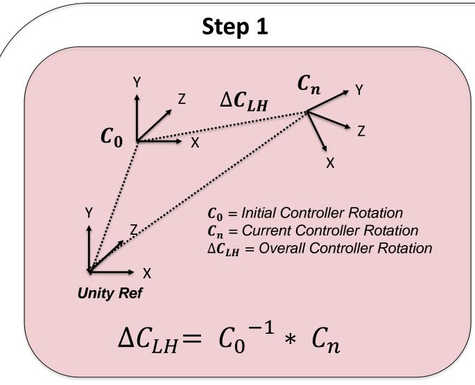
Controller trigger is pulled resulting in  $C_0$  being recorded. Each subsequent Unity frame overall rotation  $\Delta C_{LH}$  is calculated in the above equation.  $C_0$  and  $C_n$  are quaternion rotations relative to Unity's world reference frame
