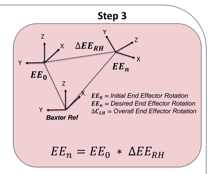
The desired quaternion  $EE_n$ , describing rotation from Baxter reference frame to the desired position, is calculated using the above equation.  $EE_n$  and  $EE_0$  are quaternion rotations relative to Baxter's Base reference. This is used in an IK solver to find joint angles for robot arm
