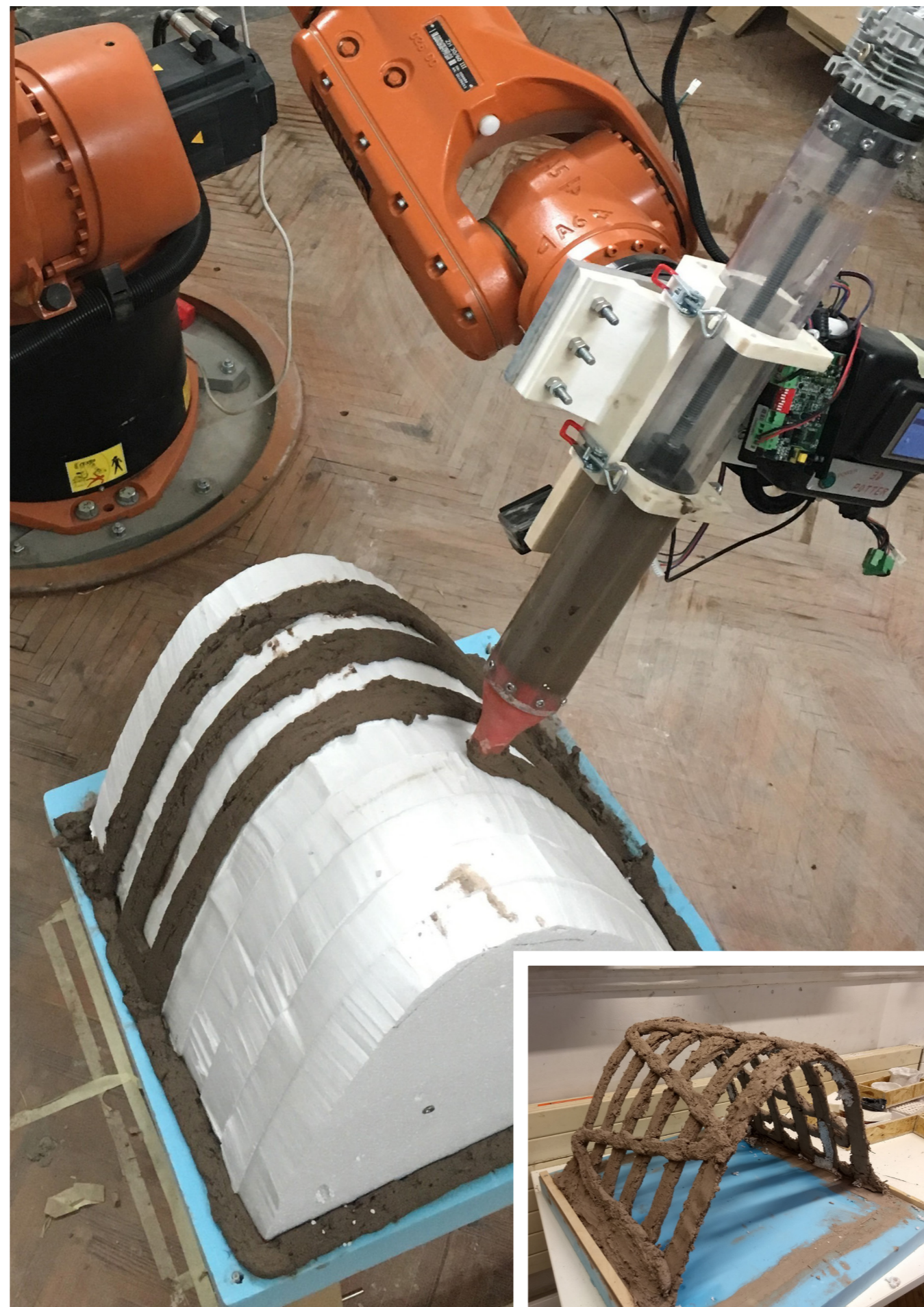
Robotic 3D printing with a mold
