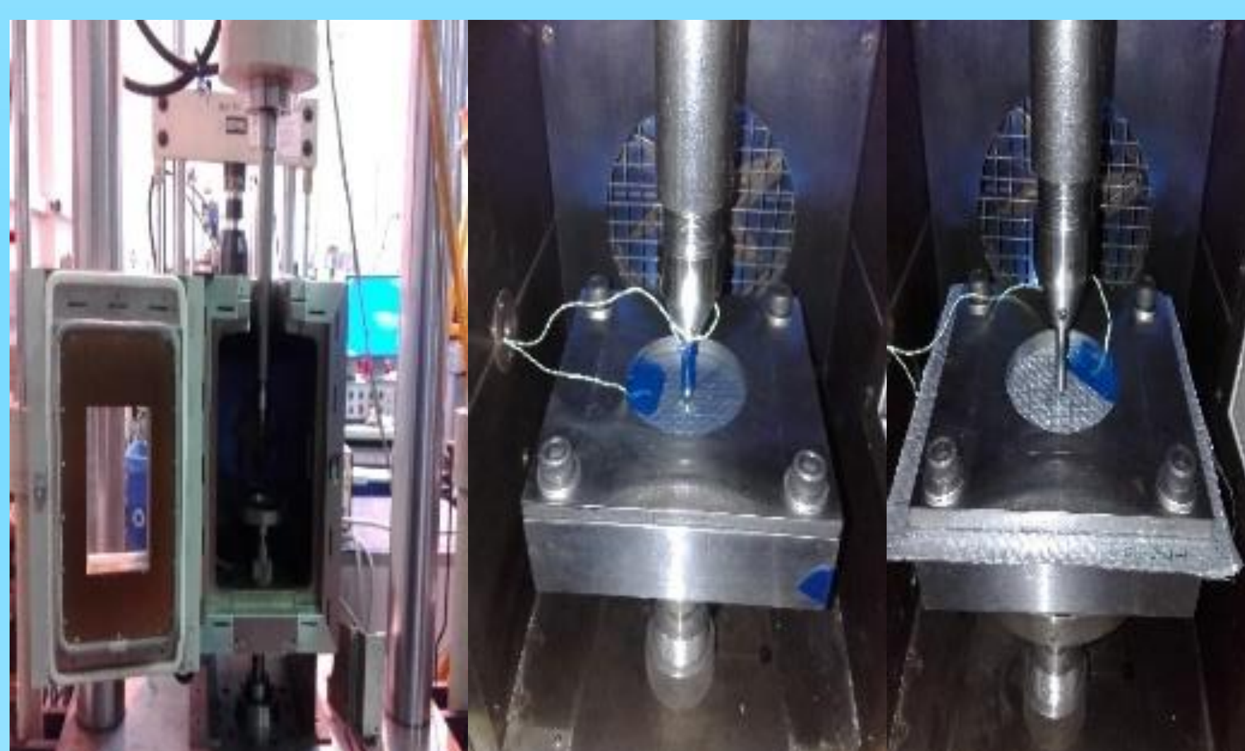
Figure 2. Single and Multiple Indentation Forming
