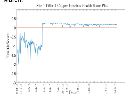
Figure 4: Health Score Plot – Copper Gearbox
